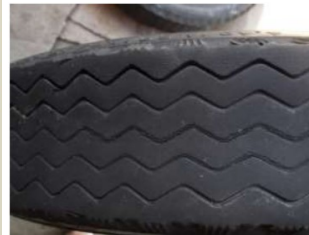
Two tires (rollers). They can be used for rolling your A around in the garage. One is worn. For the second tire, it appears that the tread seam is coming apart.
