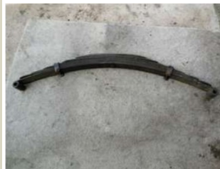
Front spring and 10 leaf rear spring. The front spring is marginal. I noticed the difference when replaced. The rear spring is good. I do not notice the difference, but the eye to eye length was 1/2 tighter on the new spring.
