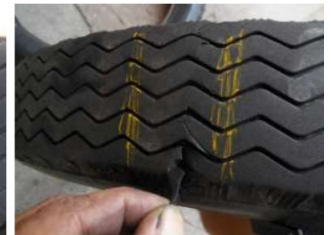
Two tires (rollers). They can be used for rolling your A around in the garage. One is worn. For the second tire, it appears that the tread seam is coming apart.
