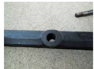
Front axle. On one of the spring perch mount holes is slightly elongated.
