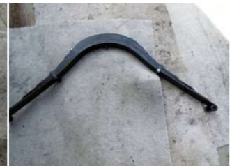
Front spring and 10 leaf rear spring. The front spring is marginal. I noticed the difference when replaced. The rear spring is good. I do not notice the difference, but the eye to eye length was 1/2 tighter on the new spring.
